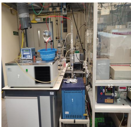
Figure 6 - Reactor assembly: 1 - Oven; 2 - Reactor; 3 - Adaptor; 4 - Collector; 5 - Condenser; 6 - Volumetric balloon; 7 - thermoregulator; 8 - Thermocouple; 9 - Temperature's display: 9.1 - SetPoint Temperature; 9.2 - Reactor's temperature; 9.3 - Programming buttons; 10 - Oven's temperature
